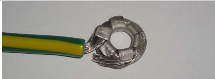
Figure 3.2: Crimping Of Star Lug For Incoming Protective Earth
